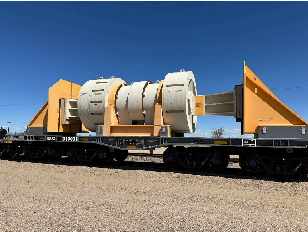
DOE's Atlas railcar, designed and tested to transport spent nuclear fuel.
