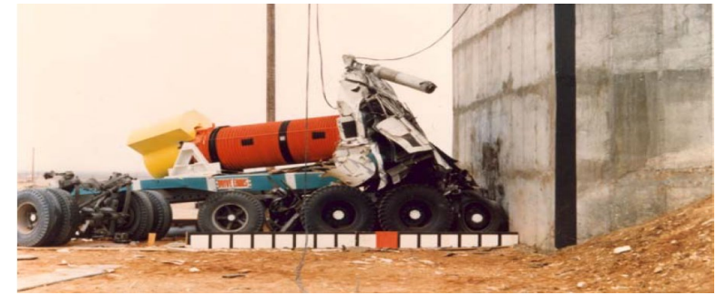
Truck tractor-trailer with SNF shipping cask. (4)
