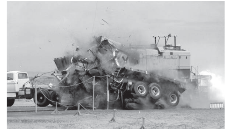
Locomotive impacting a tractor-trailer system. (4)
