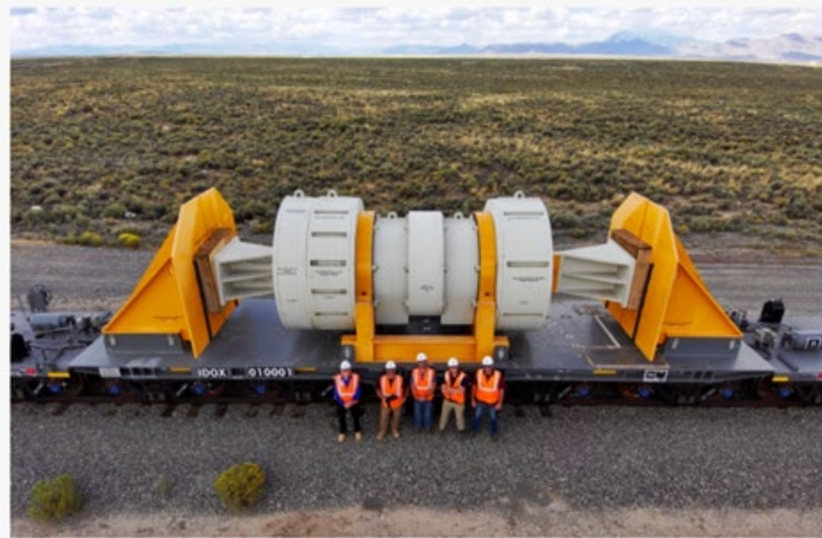
Aerial shot of the Atlas railcar carrying a test load simulating a shipment of spent nuclear fuel. U.S. Department of Energy photo
