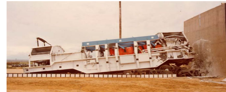
SNF package mounted in a railcar. (4)
