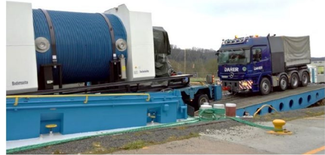
Fig. 8. Loading of cask type CASTOR ® 440/84 mvK at the berth of NPP Obrigheim.
