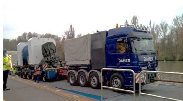
Fig. 12. Unloading Road Trailer with cask from river barge at the RORO berth of NPP Neckarwestheim.
