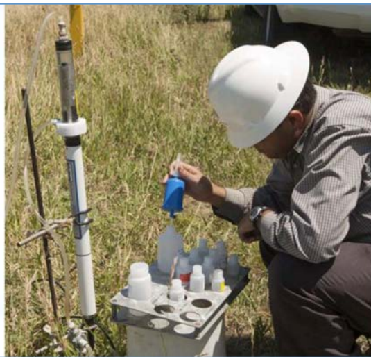
Shallow Groundwater Sampling
