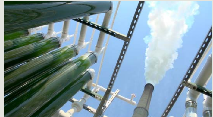
U of Kentucky pilot-scale photo- bioreactor tubes
