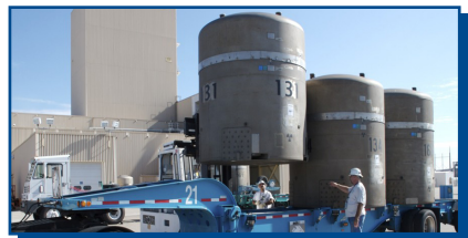
Above: An empty TRUPACT-II is loaded onto a trailer. The TRUPACT-IIs is one of several containers sent to the generator sites empty and returned with transuranic waste for disposal.
