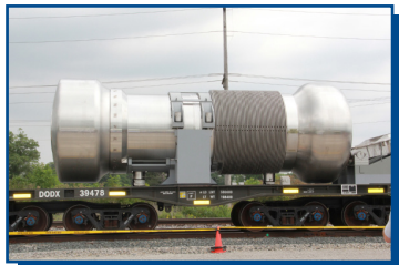
Above: The M-290 used to transport spent nuclear fuel from Navy's nuclear propelled aircraft carriers.
