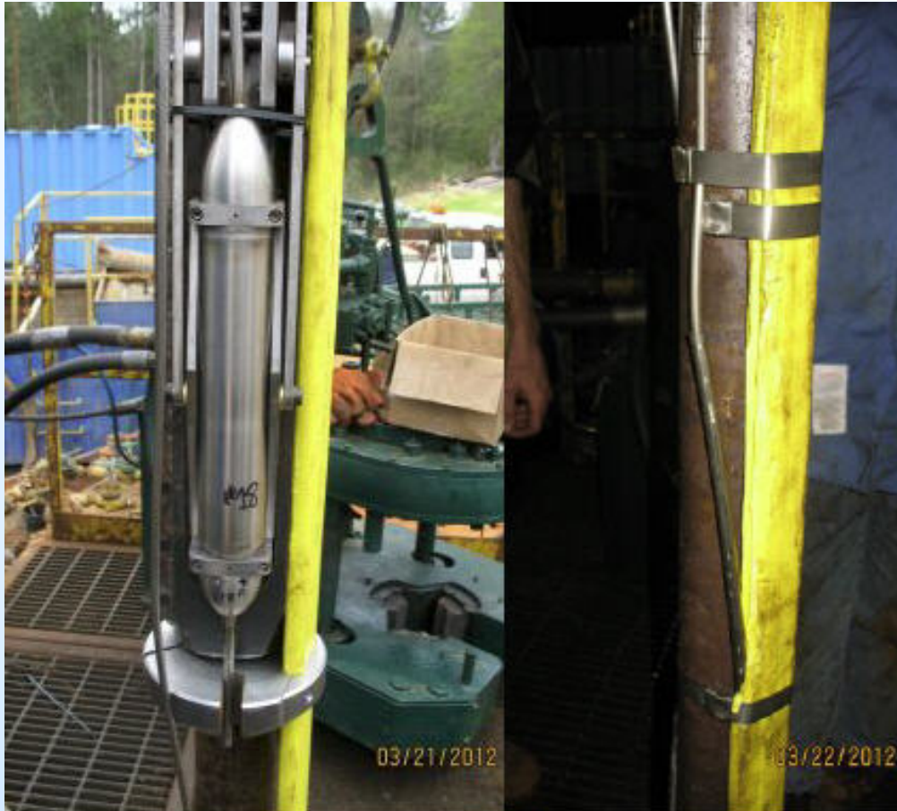
Deployment of the Modular Borehole Monitoring (MBM) Conventional geophone array (left) and yellow flat pack containing the fiber optic based DAS array (right)
