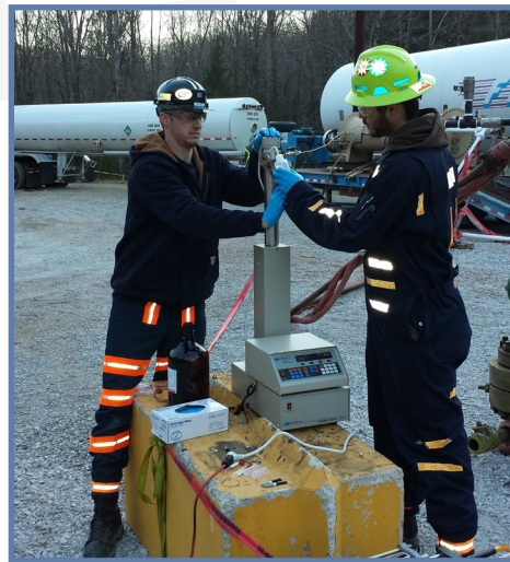
Perfluorocarbon tracers are injected with the CO 2 stream as part of the monitoring, verification, and accounting program at the site in Morgan County, Tennessee.
