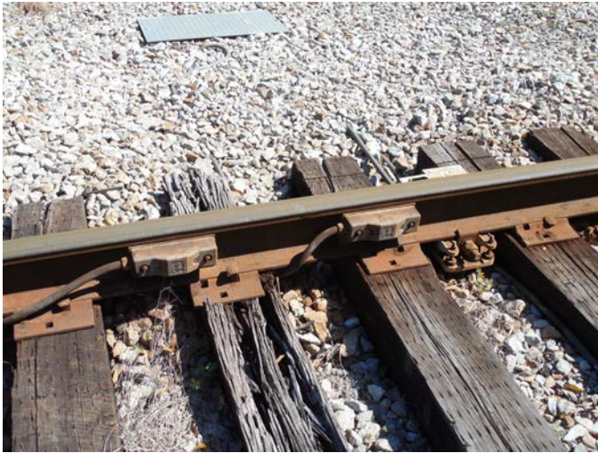
Wheel Detectors (count # of axles, determine speed, open shutter for hot bearing detector)
