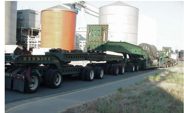
MP187 Transportation Cask Heavy Haul to Rancho Seco
