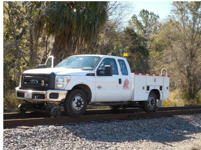
Hi-Rail Vehicle Used for Track Inspections
