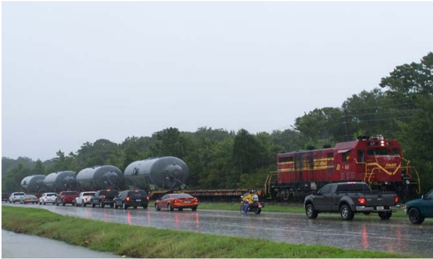
Four Moisture Separator Reheaters (MSRs) 300,000 lb. (each) 51' long x 14' diameter (July 2009)
