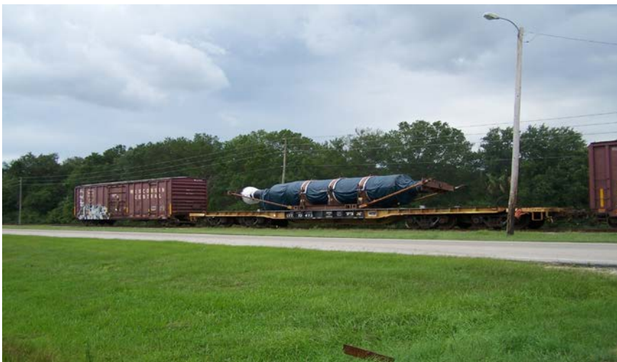
Generator Rotor 395,000 lb. 50' long x 8' diameter (October 2009)
