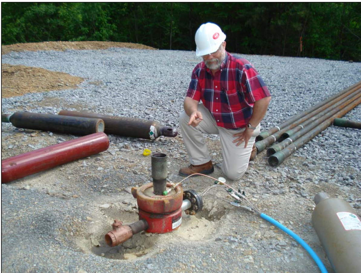
Dr. Jack Pashin, GSA, explaining the pressure gauges and gas sampling lines at the 1-South monitoring well.
