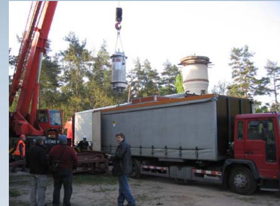
Casks of HEU spent nuclear fuel being loaded for transportation from Latvia back to Russia, May 2008
